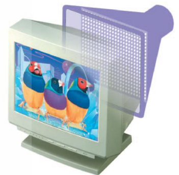
Figure 2.23: CTR screen coated with tiny phosphor dots
